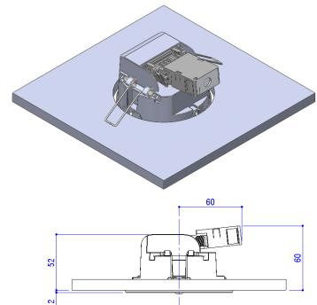
The movement detection area is rectangular with the widest view aligned with the springs and the axis along the ETAP logo and sensor openings. The sensor should be mounted in an area with much daylight (if present) and since it is the Bluetooth connection point also near the area where it is most likely someone will be sited to control the lights via the smartphone App.
